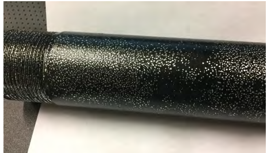
Contamination of the surface - bad pretreat.
